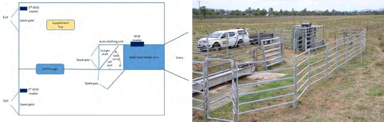
Figure 1: a) Diagrammatic representation of the ALMS unit and compound and b) The ALMS unit and compound during the training period.
