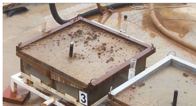
Above: Plot with a Full Stop installed in the centre for leachate collection.
