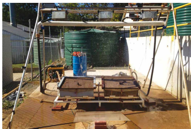
Above: Rainfall simulations on sugarcane soil at Landloch's Toowoomba soil laboratory. Run-off and leachate water samples were collected and sent to an external laboratory for analysis.
