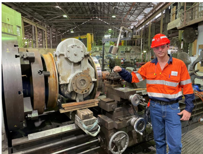
First-year fitting and turning apprentice Liam Di Bartolo inspects loco wheels being machined at the Burdekin Centralised Workshop.
