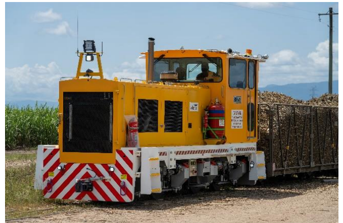
Brisbane was designed and engineered from the ground up for Wilmar’s cane haulage operations. It is 25 per cent more fuel efficient than the model it replaces.
