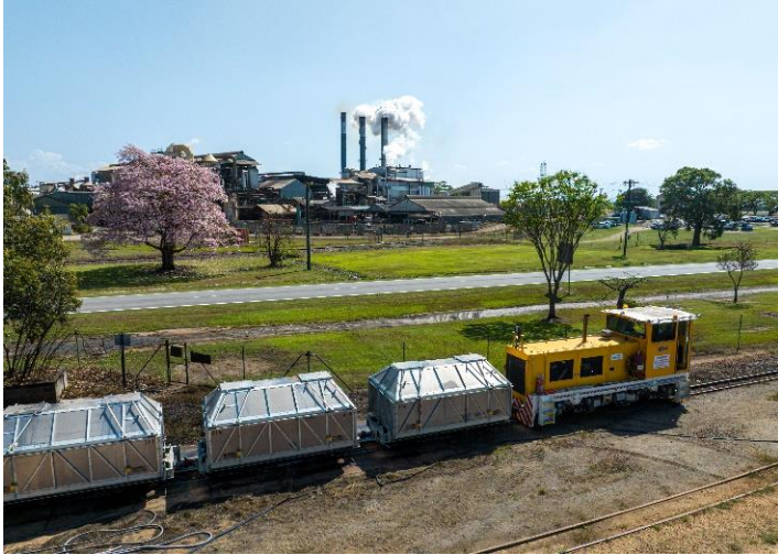
The newest loco in the Wilmar fleet, Brisbane, is being fuelled with hydrotreated vegetable oil as part of a four-week trial of renewable diesel. The product achieves a reportable emission reduction of 99 per cent.
